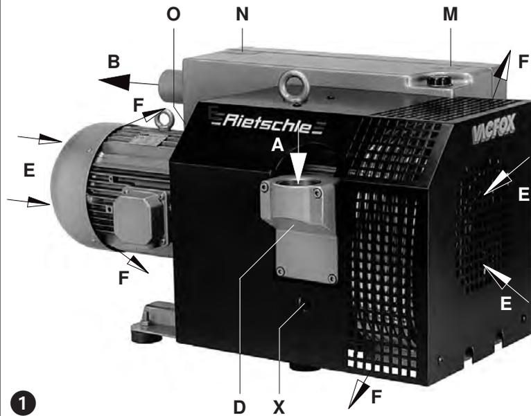
A standard built-in non return valve on the inlet of the pump seals the pump from the process when the pump is stopped. This prevents oil moving into the pumping cylinder when the pump is stationary. Excessive oil in the cylinder could cause an hydraulic lock when the pump is started and hence undue stress on the rotor blades.
